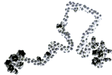
Graphical representation of a triblock SBS molecule: two polystyrene blocks connected by a polybutadiene block.
