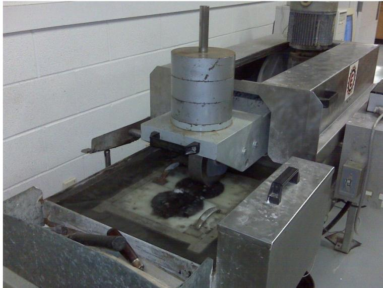
**Figure 2.3 Hamburg Wheel-Tracking Device**
