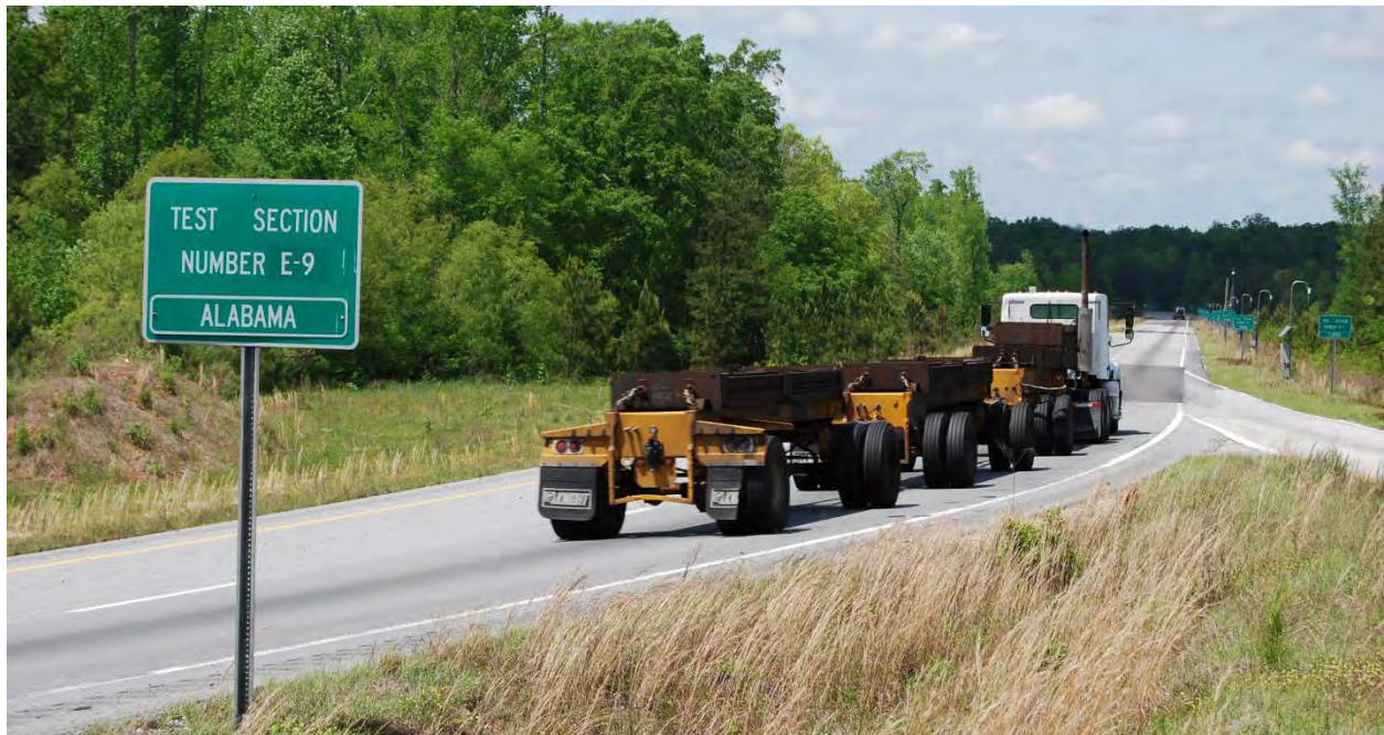
Figure 1.4 One of the Heavily Loaded Triple-Trailers used for Accelerated Loading on the Test Track
