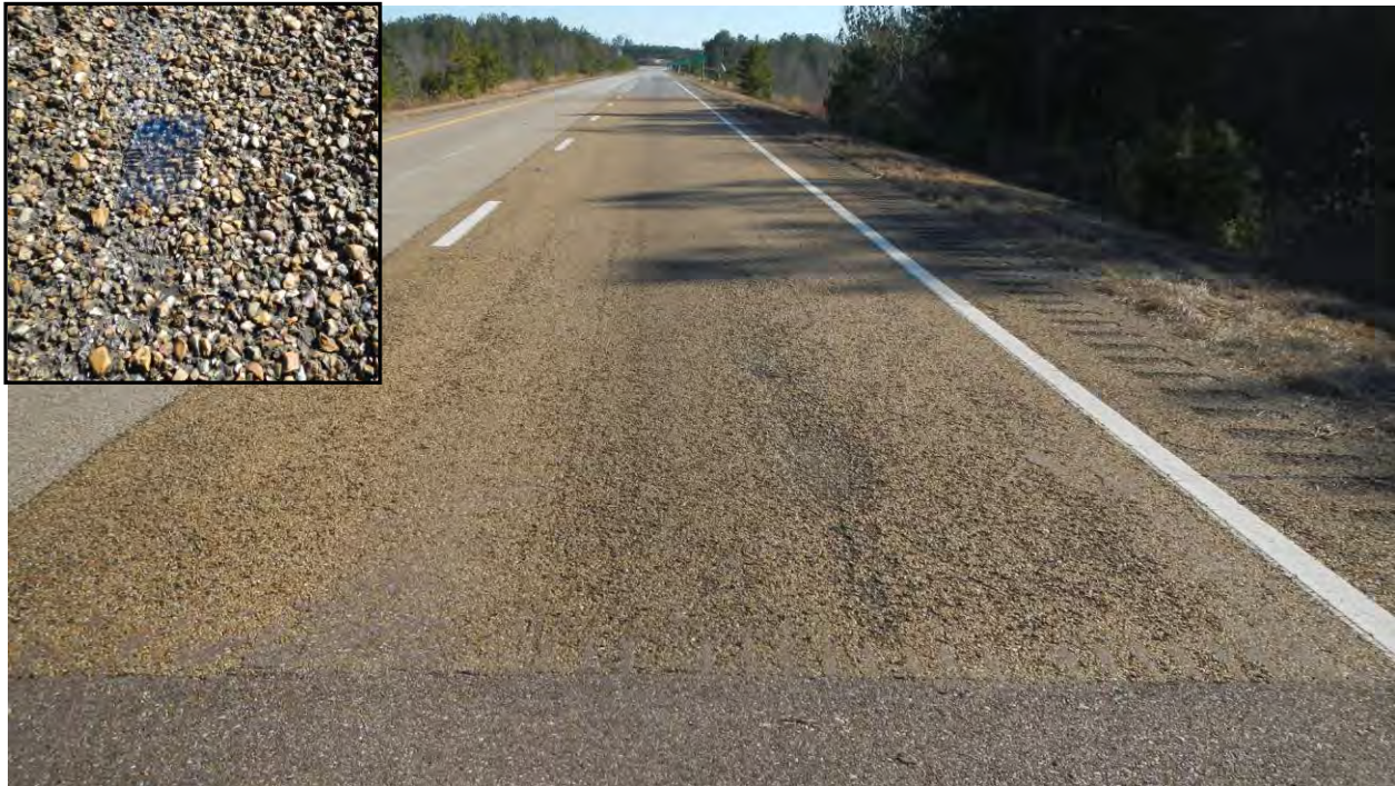
Figure 2.5 Photograph of the Initial Part of the Gravel OGFC Test Section after Two Cycles
