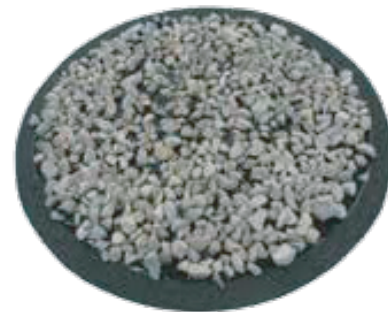
Figure 2 - Kraton D1192-Modified CRS-2P Emulsion Sweep Test Pad - Post-Sweep
