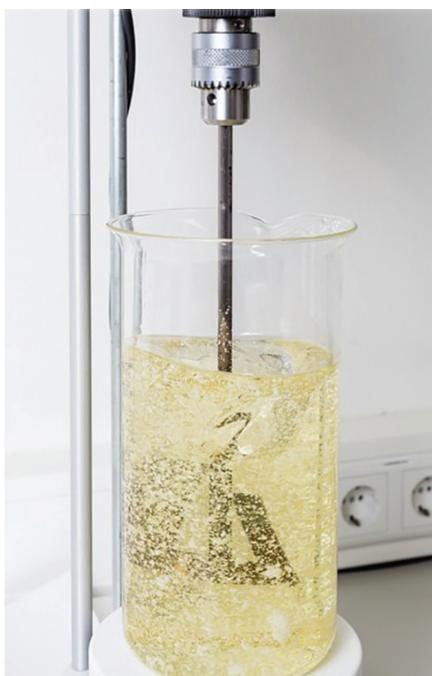
Mixing under high or low shear
