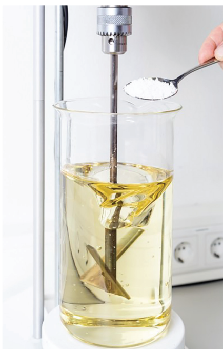
Addition of Ellamera polymer to warm oil
